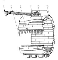
executed with automatic tools which insure long duration. The spiral is uniformly distributed within the circuit which is realised by a mosaic of ceramic blocks. This solution guarantees a perfect distribution of the heat
