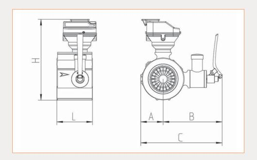
The pressure loss of the MQM Quantometer is minimized through a fluid dynamically optimized inlet diffusor, very low manufacturing tolerances and the high precision, low friction ball bear-ings. The optimized flow conditions allow a minimal straight inlet pipe of >/= 3 DN. If the instal-lation conditions allow or in case of severe flow perturbations acc. to OIML a straight inlet length of >/= 5 DN is recommended."
