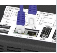
Two Ethernet 10/100/1000 Mbit ports on the rear side of the operator panel are available. ETH1 and ETH2 are internally connected to CPU through a Gigabit switch.
