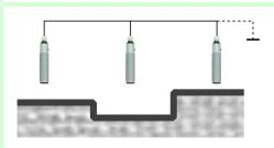
In this working mode the sensors measure in a chain. All sync terminals (SYNC) must be connected to each other and also to ground (-Vdc). Power up the system and after 5 seconds disconnect the ground.
