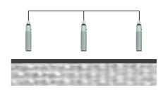
In this working mode all the sensors measure simultaneously. All sync terminals (SYNC) must be connected to each other and the system must be powered.
